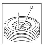
When the tire has been lowered, tilt the retainer (D) at the end of the cable so it can be pulled up through the wheel opening.
